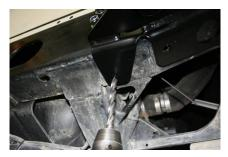
12. The top brace, must be fitted. This slides between the body and the top of the chassis.
